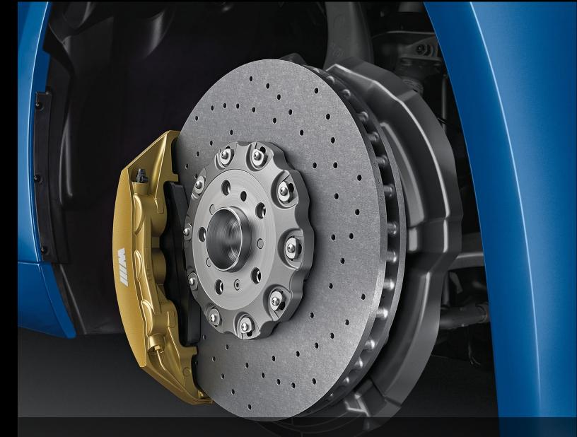
M Carbon Ceramic Brakes made from innovative Carbon Fibre compound materials make braking even more direct and improve response to heat build-up?
